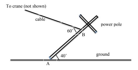
The centre of mass of the pole is one third of its length from the base and the cable from the crane is attached at point B, 9.50 m from the base of the pole. If the crane has stopped lifting and the pole is at rest in the position shown in the diagram find,
